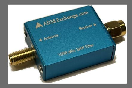
There are also filter and Filter/Low noise amp combos for 1090
